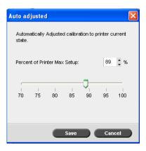
Note that this one slider affects all the four process colours, which cannot be adjusted individually. You might have to settle for a compromise based on all four toners. After calibration, a new density curve is automatically saved on the RIP for both "Normal" and "Saturated" print. You can test both and see which ones give you the best density values. This setting must thereafter be set as default for the relevant print queues.
