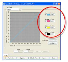
In this window you can type in the desired density values from PrintSpec. Note that the calibration routine on EFI Fiery RIPs are always Status T, so even if you use Status E for offset work or in PrintSpec, you must use a Status T Standard in PrintSpec to obtain the target values. There is a big difference in readings of yellow ink and toner between Status T and E, so this is important. When you later measure prints in PrintSpec you are free to use both Status T and E.
