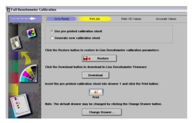
**Full Color calibration:** Run a full color calibration by the default setting. The press will be calibrated to 15 points on the TVI curve for each ink.
