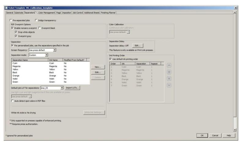
Make sure ICC colour management is off, by setting the CMYK Input Profile and Emulation Profile to None:
