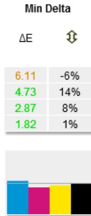
The % numbers shows you how the density should be adjusted. In this example, cyan should be brought down 6%, while magenta should be brought up 14% and yellow 8%. The black ink can be left as it is.
