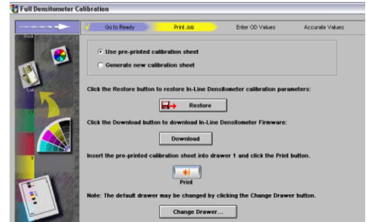
**Full Color calibration:** Run a full color calibration by the default setting. The press will be calibrated to 15 points on the TVI curve for each ink.
