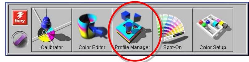
The Profile Manager window that opens is used for managing the ICC profiles on the RIP. You can use a standard profile that was delivered
